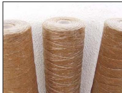
**Figure 8.** Cartridge Filters used during DO and Filtration Testing
