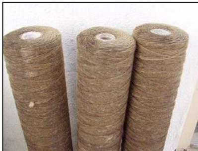
**Figure 7.** Cartridge Filters used during ClO<sub>2</sub> and Filtration Testing
