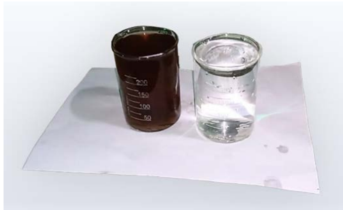
Figure 1: Water quality comparison (Wastewater on the left and RO effluent on the right)
