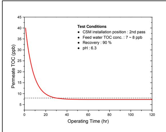
TOC reduction in CSM UPW products used in the 2<sup>nd</sup> pass ultrapure water system. Rinse down time may vary according to the feed water conditions.
